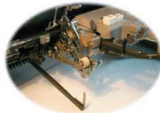
When a handle is pressed, the "finger" raises the slug, which is seized by the rectangular sleeve just below the little white ceramic roller. After printing, the slug is released by a push from the ceramic roller and drops back into the tray.
