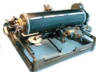
The character tray is removed, revealing the "finger" that raises the character slugs.
