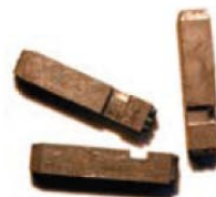
When a handle is pressed, the "finger" raises the slug, which is seized by the rectangular sleeve just below the little white ceramic roller. After printing, the slug is released by a push from the ceramic roller and drops back into the tray.
