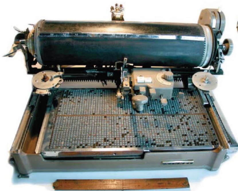
The Nikkei Master with platen, typing assembly, and character tray. 12-inch ruler shown for scale.
